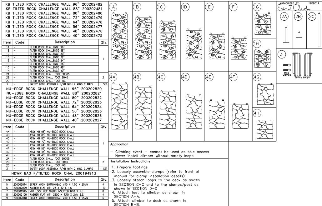
6. Tighten all hardware and install clamp drive
