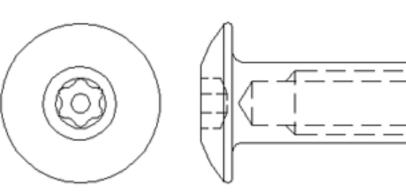
200001954 BARREL NUT M10 X 1.50 (12.70 DIA x 32mm)
