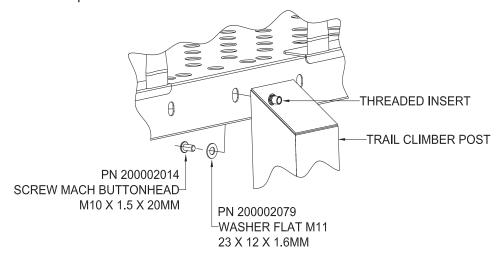
6b. Tighten all hardware and install clamp drive pins.
