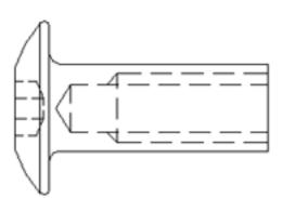
200001954 BARREL NUT M10 X 1.50 (12.70 DIA x 32mm)
