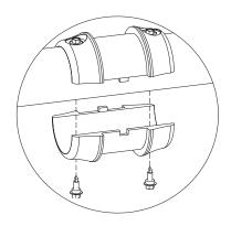
3d. Place steel hanger around plastic collar; apply Vibra-Tite Threadlocker to end of tamper proof bolt; attach H-shackle to hanger via tamper proof bolt; tighten all hardware.
