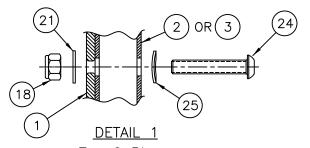
Typ 6 Places (handrail to step attachment)
