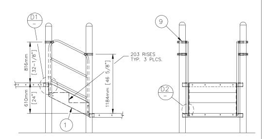
DETAIL 1:5 STEP TO DECK ATTACHMENT DETAIL TYP. 4 PLCS. BOTH ENDS 8 DETAIL D2 1:5
