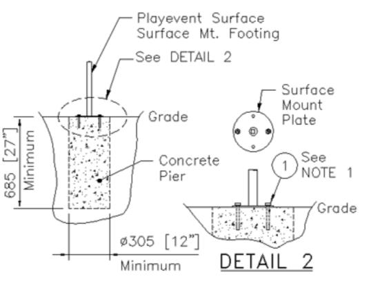
NOTE 1: Two per plate, diagonally located.
