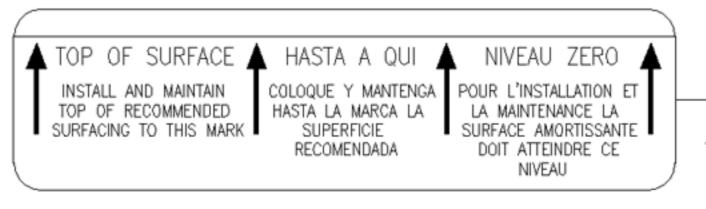
The sticker shown here has been provided to assist with the maintenance of your ground cover. After installing the ground cover, these stickers should be placed on the post by the installer (as shown). Peel the backing away from the sticker and attach it to the post so that the line is level with the top of your ground cover. As erosion or compaction of surfacing occurs, the line will be visible. This will indicate that it is time to add material to your surfacing.
