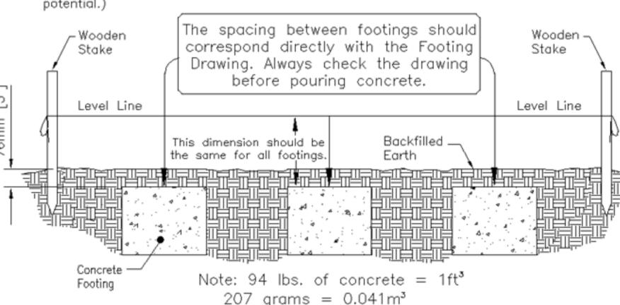
If installing with the Inground method, you must always backfill footings with at least 76mm[3"] of earth after concrete has cured (not shown).
