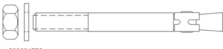
200001776 ANCHOR CONCRETE WEDGE M10 x 1.5 x 100mm
